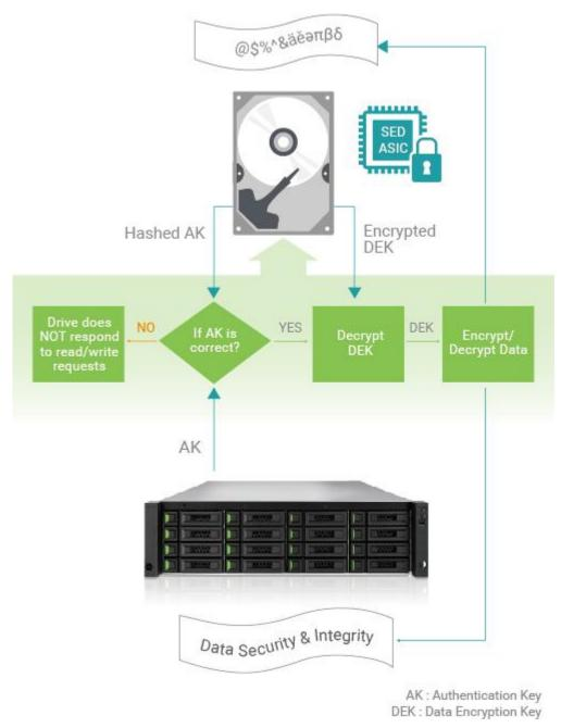
Figure 1 SED Operation Process
